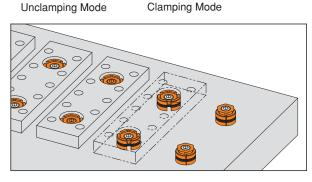
Example of application where two I.D. Holding Clamps are used.
